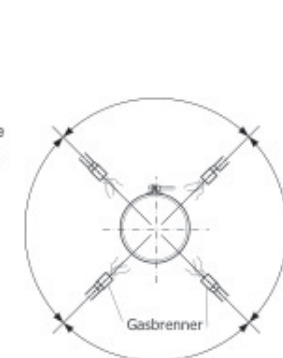
Figure 2-4: Test set-up "Joint flame test" from DN 200 to DN 300
